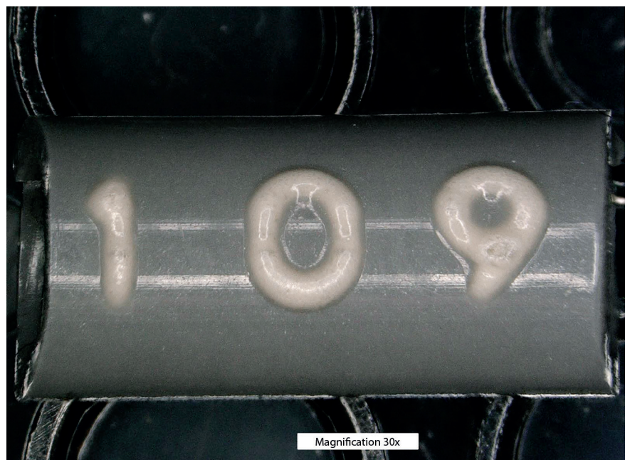
Fig. 4. The formation of white foam ensures a good contrast on the dark background, but also causes a significant modification of the component's surface (© Fietz Polychromos)
